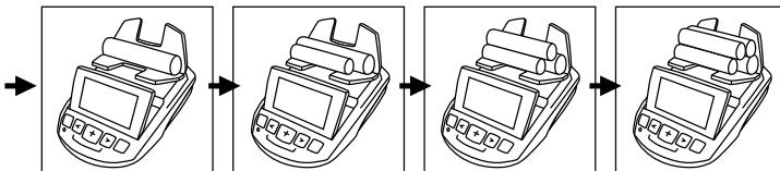
max. weight = 1 kg; at the end remove ALL coin rolls from the scales together
